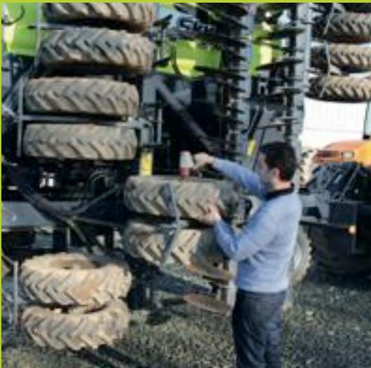
**The roller has twin-mounted wheels equipped with scrapers. Each pair is staggered.**
